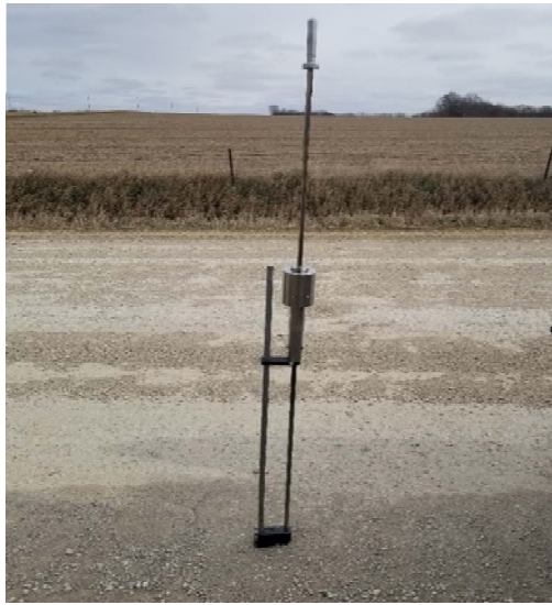
Figure 8 Kessler K-1000 dynamic cone penetrometer
