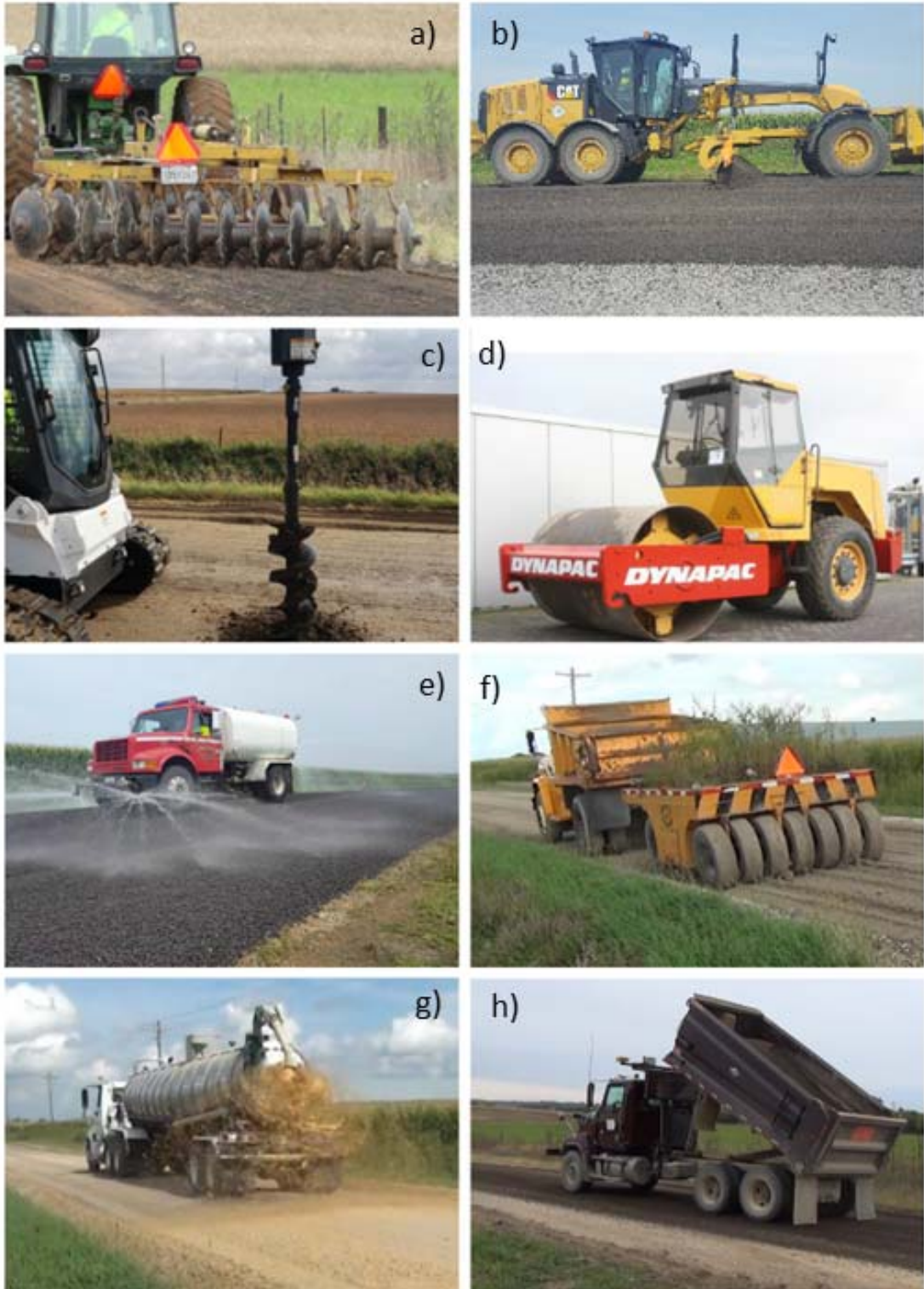
Figure 20 Equipment used for mechanically stabilized sections a) disk plow harrow b) motor grader c) power auger d) vibratory compactor e) water truck f) rubber tire roller g) self-unloading tanker trailer spraying clay slurry h) dump truck
