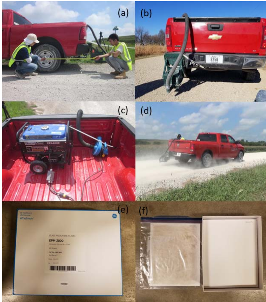
Figure 13 (a, b, and c): Dustometer test setup, (d): a test conducted on the granular-surfaced road test sections, (e): EMP 2000 glass microfibre filters, and (f): filter paper before and after test.
