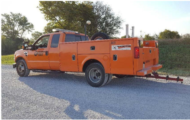
Figure 10 SN121 JILS falling weight deflectometer used in this study
